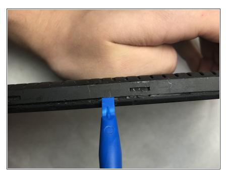
Wedge the plastic opening tool into the seam nearest to the screen surface and begin to pry off the back of the device.
