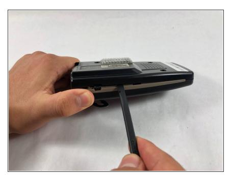
• Pry off the back panel of the radar using the nylon spudger.
