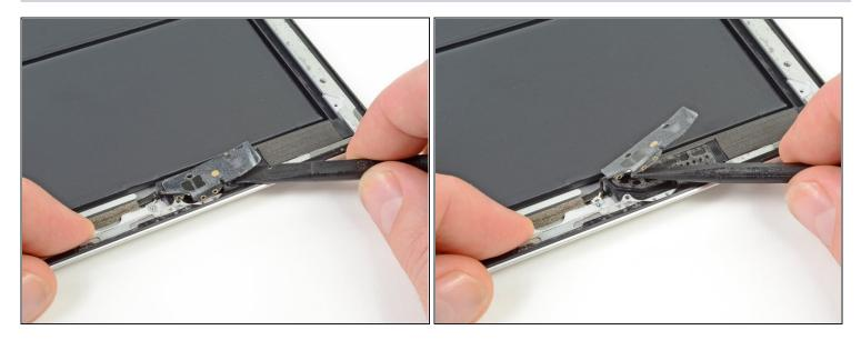
• Use the flat end of a spudger to loosen the foam adhesive holding the Wi-FI antenna to the speaker assembly.
