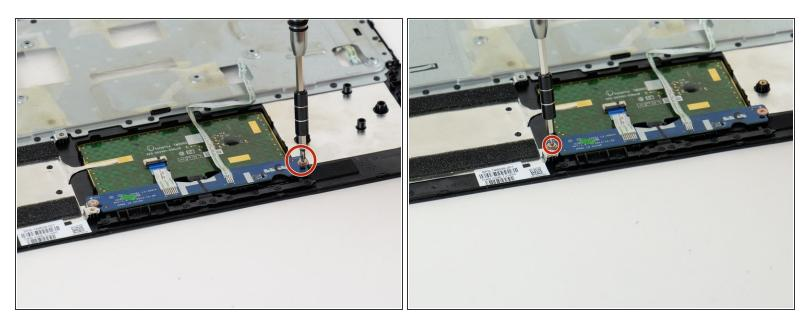
• Remove the two Phillips screws securing the button board.
