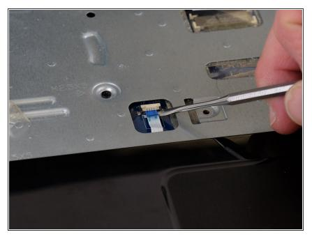
• Now disconnect the touch pad ribbon cable by lifting the connector.
