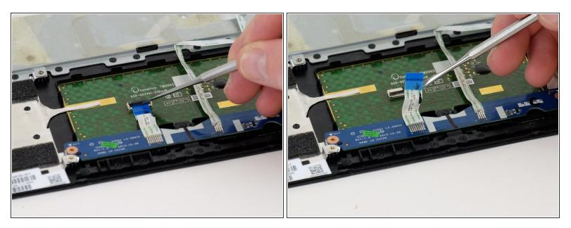
• Release the cable connected to the button board.
