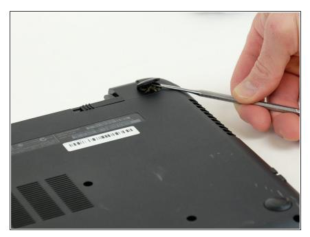
• Using the spudger, remove the two rubber feet that are located near the battery.
