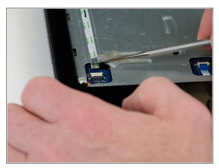
• Disconnect the power button ribbon cable by lifting the connector.
