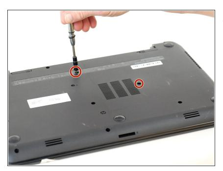
• Remove the two 5 mm screws with the Phillips #00 screwdriver.
