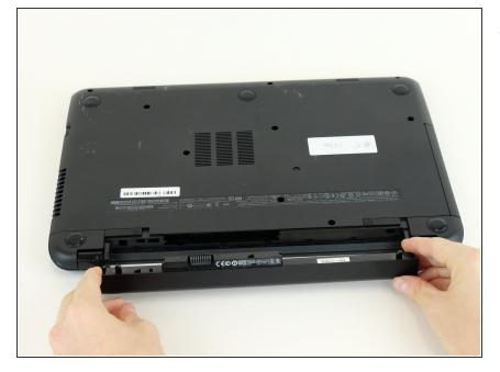
• Pull on the battery to remove.
