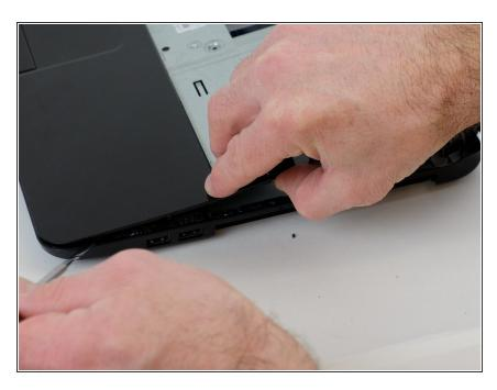
• Lift up on palm rest, while working the spudger around the perimeter.
