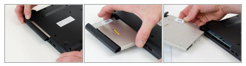
• Remove the optical drive by pulling it out by hand.
