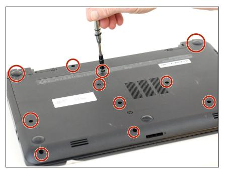
Using a Phillips #00 screwdriver, remove all the 5 millimeter screws located on the bottom of the laptop.
