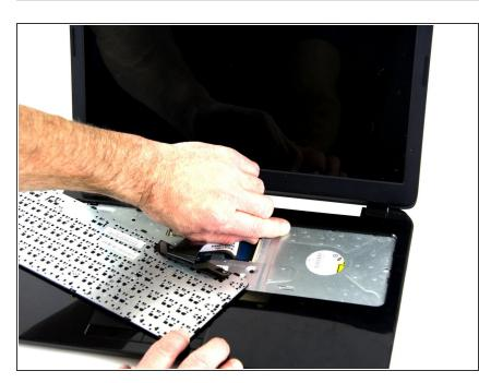
Remove the ZIF connector that connects the laptop to the keyboard cable.
