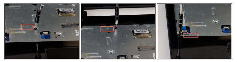
Remove the screws indicated by an arrow stamped into the metal.
