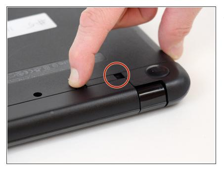
Slide the latch towards the center of the laptop so the unlock emblem appears.
