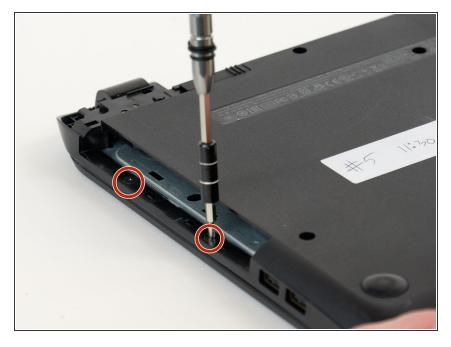
• Remove the two Phillips screws inside the optical drive housing.
