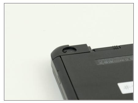
Now remove the two Phillips screws that are located below the rubber feet.
