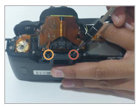
Using a PH000 screwdriver bit, remove the 2 black screws circled in the picture, which are both 8 mm in length and 1.5 mm in diameter.
