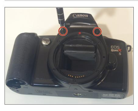
Using a Phillips #000 screwdriver, remove the two black screws shown in the picture that are both 6 mm in length and 1.25 mm in diameter.
