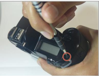
Using a PH000 screwdriver bit, remove the three black screws shown in the two pictures that are all 4 mm in length and 1 mm in diameter.
