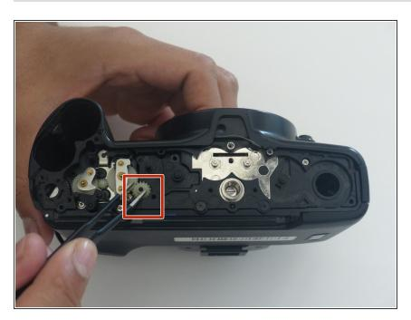
Remove the gear with tweezers or fingers.
