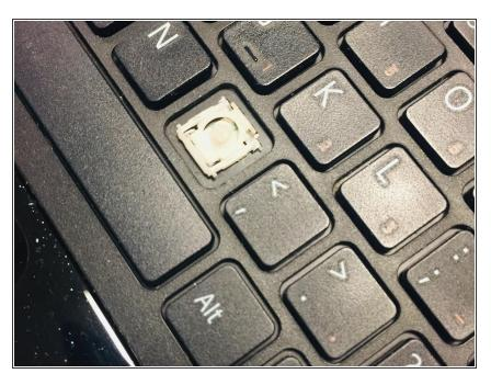
After the key is removed, you should be able to see the part underneath the key where it can be replaced.
