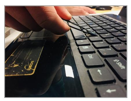
Carefully lift the key piece upward to remove it completely.
