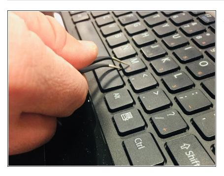
Use the tweezers to get under the key piece on the keyboard as shown in the picture.
