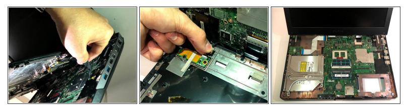
• Remove the ribbon connectors that connect the keyboard to the motherboard. The keyboard should now be completely disconnected from the laptop.
