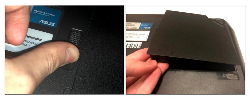
• Make sure the computer is off and turn it over on its back. Push the slider all the way back until the compartment for the battery opens. Remove the battery and place it aside.
