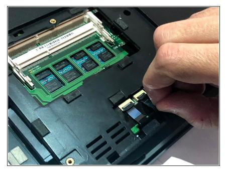
When the back panel is removed, disconnect the blue and black ribbon connectors exposed from the back panel.
