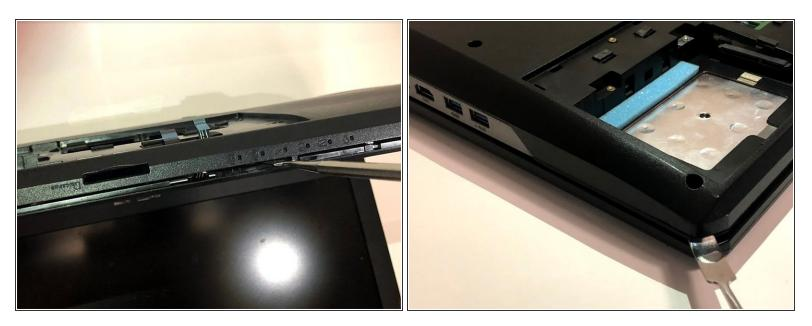
Begin to pry the keyboard off of the laptop with the pointed metal spudger.
