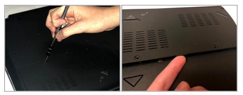
• Find the panel on the back of the computer. Use a Phillips #0 screwdriver to unscrew the 2 4.2mm screws on that panel. Next, lift up the panel at the indent and place it aside.
