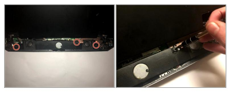
Use a Phillips #00 screwdriver to unscrew 3 screws on the audio board.
