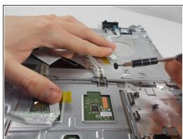
Use a 1 1/2 mm flathead screw bit to remove the two black screws at the top of the panel.
