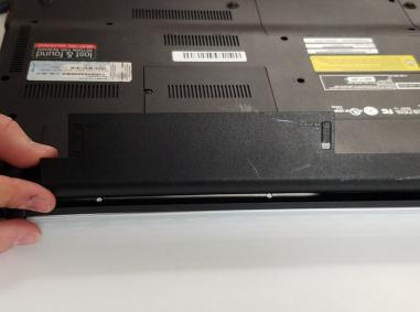
Hold the switch that says "Release" to the open position while pulling up on the side of the battery with the groove. Once the battery is flipped up, it can easily be removed. To reassemble your device, follow these instructions in reverse order.
