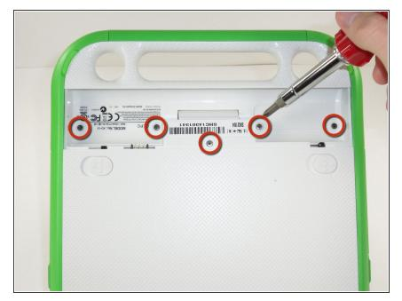
Using the Phillips screwdriver, unscrew the 5 size M2 x .4 x 4mm screws underneath the battery.
