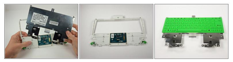
• Separate the keyboard from the touchpad. Nothing holds the keyboard and touchpad together, so they should separate easily.
