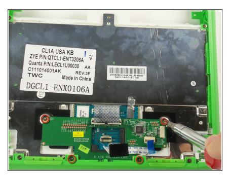
Using a Phillips screwdriver, unscrew the 4 size M2 x .4 x 4mm screws in the corners of the circuit board.
