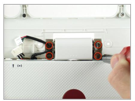
Using the Phillips screwdriver, unscrew the 4 size M3 x .5 x 5mm screws holding the metal to the rest of the laptop.
