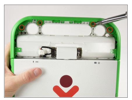
Unscrew the 4 size M2 x .4 x 4mm screws that are connected to the green plastic.
