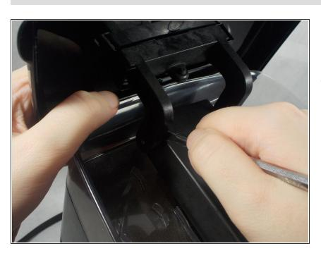
Repeat the last step on the other hinge, making sure to keep a firm grasp on the lid as it comes off to avoid dropping it. To reassemble your device, follow these instructions in reverse order.
