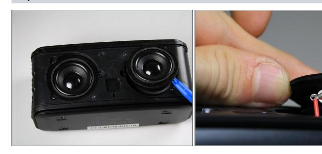
Use the Plastic Opening Tool to gently lift the speaker enough to see the connected wires.
