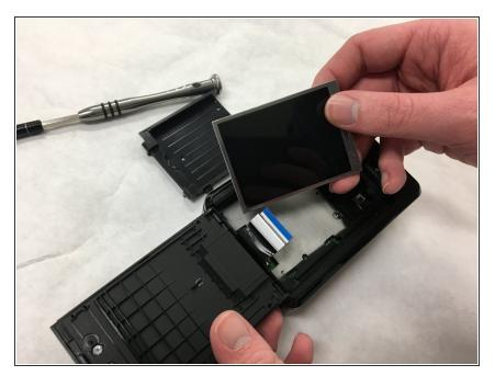
Once the panel is removed, the malfunctioning screen will slide out and can be replaced.
