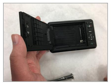
• Flip the camera to back side up and open the paper/screen door.
