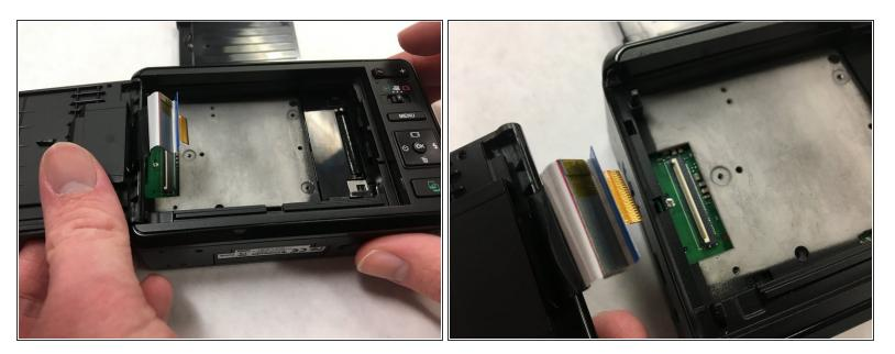
Gently pull the ribbon away from the logic board. This will allow the screen to separate from the rest of the camera.
