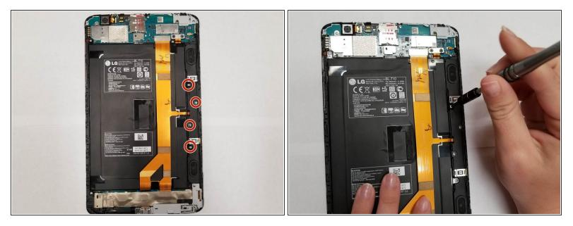
• Remove the 4 1.5 mm screws holding the speakers in place.
