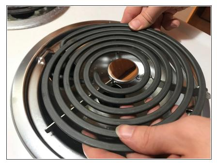
Gently set the burner back onto the stovetop.
