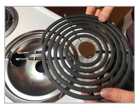
Dispose of your old burner and take your new burner out of its packaging. It is ready to attach.
