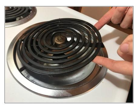
Detach the stove burner by gently lifting it up (you can use a flat head screwdriver to lift the burner if it is stuck).
