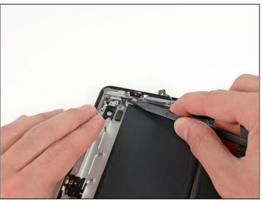
• Continue sliding the tip of the spudger toward the top of the iPad, releasing the adhesive.
