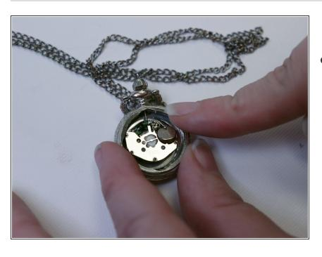
Replace the old battery with a new one by carefully sliding it back into place until it sits flat inside of the watch.
