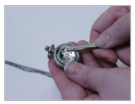
Reinsert the plastic covering into the pocket watch where it previously was by using the tweezers again until the plastic is also sitting flat in the back of the watch.
