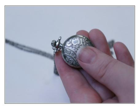
Put the cover of the watch back on by placing it and pushing it down until you hear a small click.
