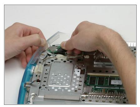
Push out the lower case rim and pull the RJ-11 board out of the computer.
