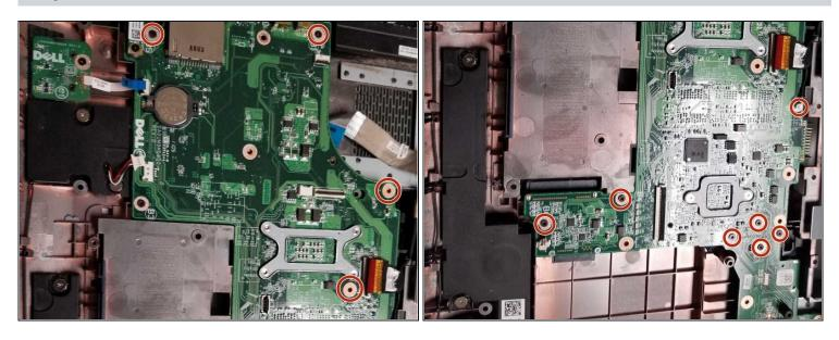
Remove all 10 screws on the motherboard using the Phillips #0 screwdriver.
