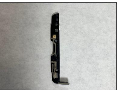
After the top and bottom screws are removed remove the top and bottom plastic pieces that were secured to the device.
