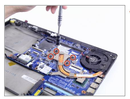
Use a Phillips #0 screwdriver to remove the four M2 x 6mm screws connecting the heatsink to the motherboard.
