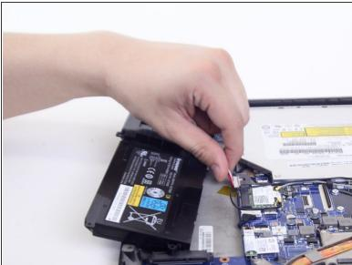
Disconnect the cable connecting the battery and the motherboard
