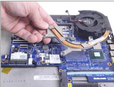
Disconnect the cable connecting the fan to the motherboard, then remove the fan and the attached fan component from the case.
