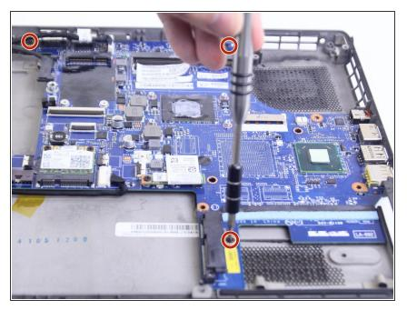
Use a Phillips #000 screwdriver to remove three M2 x 2mm screws from the sides of the motherboard.
