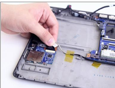
Disconnect the cable connecting the VGA connector to the motherboard. Then disconnect the cable connecting the card reader to the motherboard.
