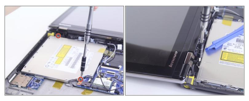
Remove the two M2 x 3mm securing the the optical drive to the device using a Phillips #000 screwdriver.
