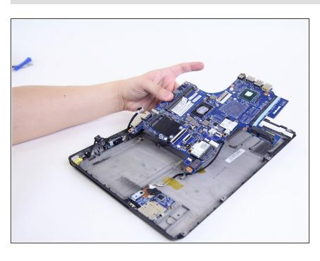
Lift the motherboard from the case and detach the cable from the back of the motherboard connecting to the DC power jack. Remove the motherboard from the case. To reassemble your device, follow these instructions in reverse order.
