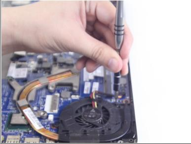
• Use a Phillips #00 screwdriver to remove the two M2 x 3mm screws from the fan.
