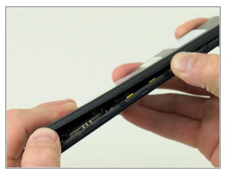
• Pry around the edges of the tablet with your fingers until you have successfully removed the back of the device.
