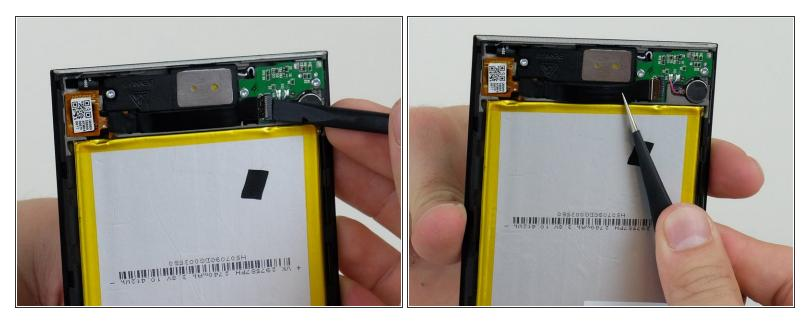
The black ribbon can be easily damaged during this step, so proceed with caution.
