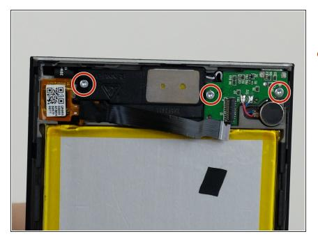
Remove all three 3mm-long silver screws using the T5 Torx screwdriver.
