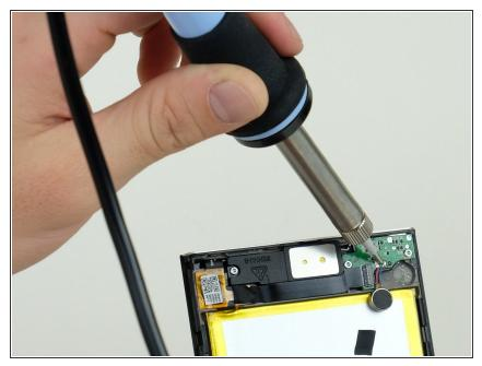
When reassembling, you will need to use the soldering iron to solder the red and blue wires back to the circuit board.
