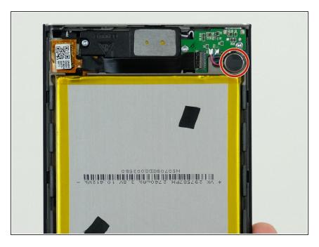
After removing the back cover, you will be able to gain access to the speaker component.
