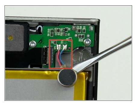
Pull the red and blue wires from the green circuit panel.
