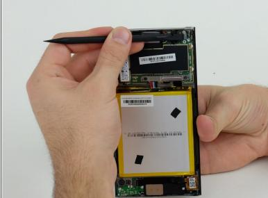
Use the flat end of the spudger to pry the ribbon holder upwards.
