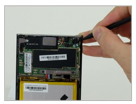
Using the pointy end of the black plastic spudger, carefully remove the black tape covering the plug.
