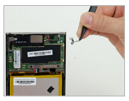
Continue pulling the black tab until you have completely removed the power button from the device.
