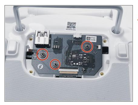
Remove the three PH0 screws securing the PCB to the remote.
