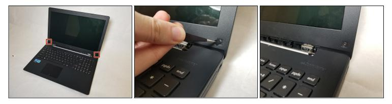
• Using <u>tweezers</u>, remove the (2) two magnetic tabs covering the screws on the screen.
