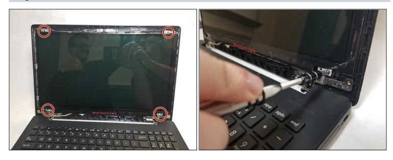
• Use a JIS #0 screwdriver to unscrew the four 3.5mm screws.
