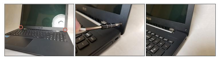
Use a JIS #0 screwdriver to remove the two 4.5mm screws.
