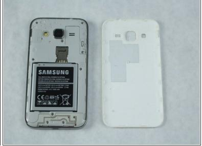
• Locate the battery near the bottom of the phone. The battery is square, flat, and is labeled 'SAMSUNG'.
