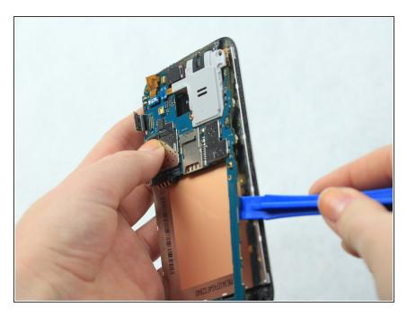
Lift the motherboard from the phone with an <u>iFixit Opening Tool</u>.
