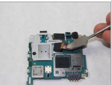
Turn the Motherboard over and disconnect the ribbon connecting the camera to the Motherboard with an <u>iFixit Metal Spudger</u>.
