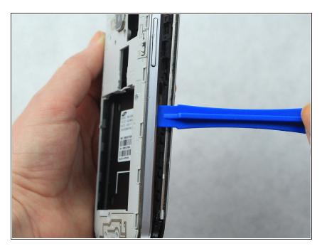
Use the <u>iFixit Opening tool</u> to pry off the midframe.
