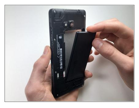
Use the plastic opening tool or your fingers to lift the battery out of the phone.
