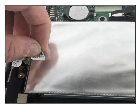
• Peel off the adhesive strap from the hard drive.
