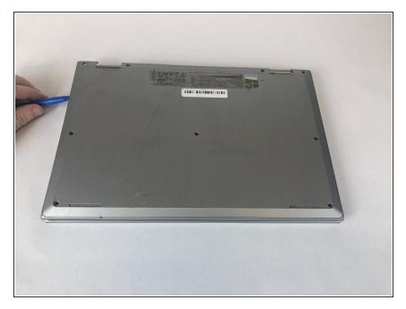
• Use a plastic opening tool to remove the cover from the computer.
