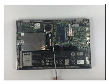
• Remove the hard drive cable from the battery.
