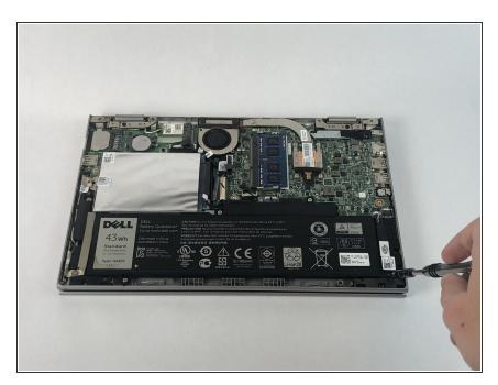
Remove the three 4.7mm PH0 screws that secure the battery to the computer.
