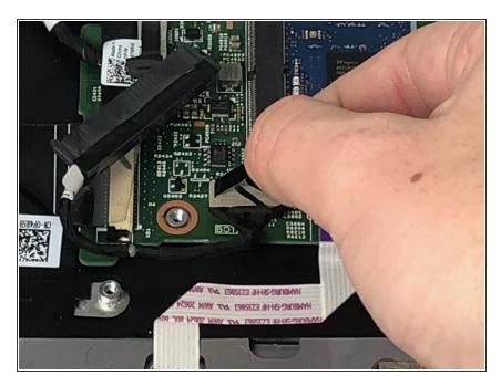
• Use pull tab to remove hard drive cable from motherboard.
