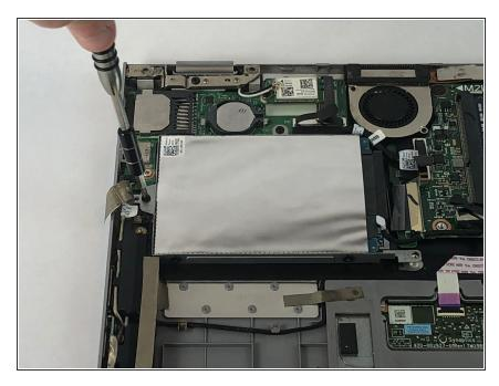
• Use a PH0 screwdriver to remove the 2 3.9 mm PH0 screws on the hard drive.
