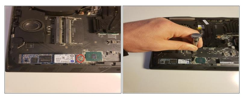
• Remove the single 1.2mm screw securing the SSD to the laptop using the JIS #0 screwdriver.
