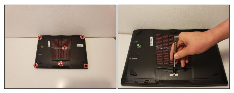
• Remove the six 1.2mm screws on the bottom plate of the laptop using a JIS #0 screwdriver.
