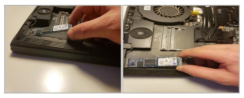
• Remove the old SSD, then insert and screw in the new one.
