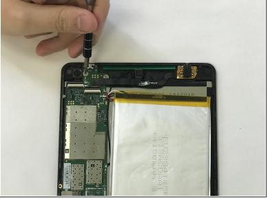
Remove the two JIS #000 screws.
