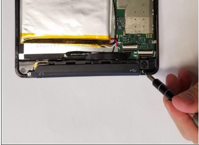
• Using a JIS #000 screwdriver, remove the two 2.5 mm screws.
