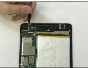
• Remove the two JIS #000 screws.
