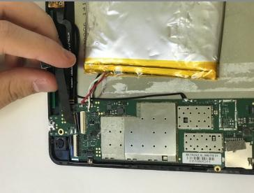
Remove all wire connections by sliding them out of the connectors.
