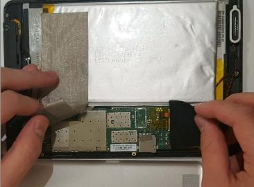
⚠ The black tape is stuck to delicate wires; remove with caution.
