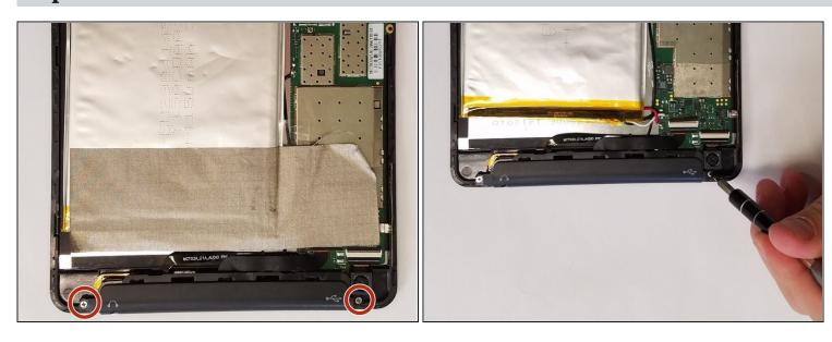
• Using a JIS #000 screwdriver, remove the two 2.5 mm screws.
