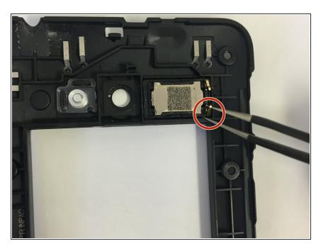
Remove speaker with standard tweezers to minimize damage, and replace.
