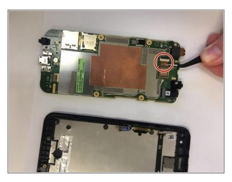
Using tweezers pull out the connector that connects the camera to the motherboard.
