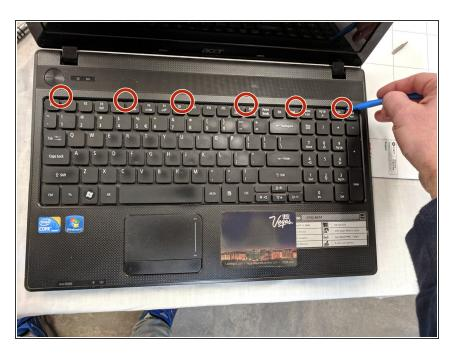
Open laptop then use the plastic opening tool to push in the 6 tabs at top of keyboard.
