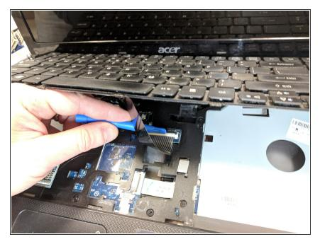
Gently lift up keyboard to access the keyboard connection ribbon. Use plastic opening tool to pop the ribbon cable lock open.
