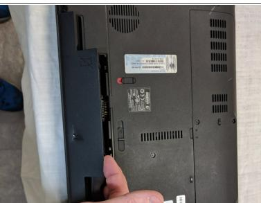
Place laptop upside down and push battery lock slider to the left to unlock. Lift battery out of case.
