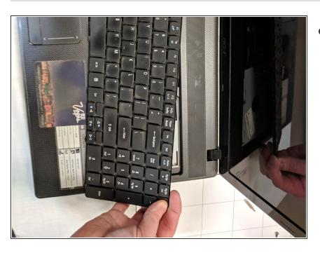
Once keyboard ribbon cable is unlocked, pull cable free and remove keyboard.
