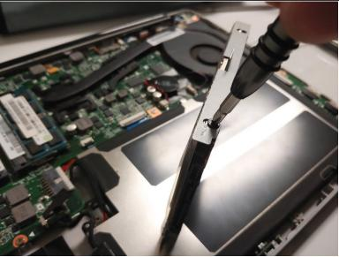
Unscrew the four screws on either side of the hard drive with the Phillips #1 screwdriver.
