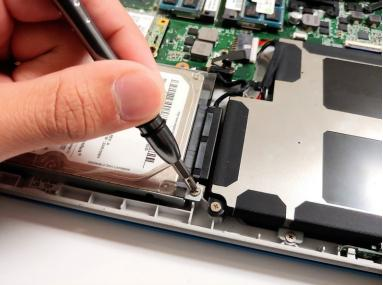
Use the Phillips #1 screwdriver to remove the three 3mm screws located on the rim of the hard drive.
