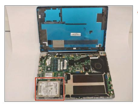
Locate the hard drive in the bottom left corner.
