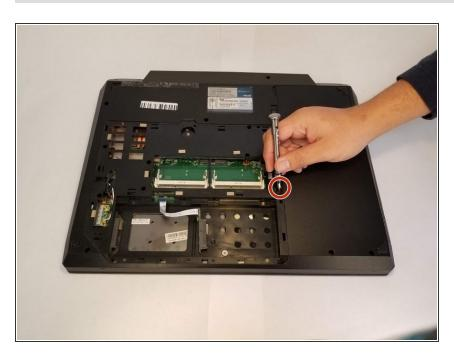
Remove the screw that is located on the right edge of the removed cover.
