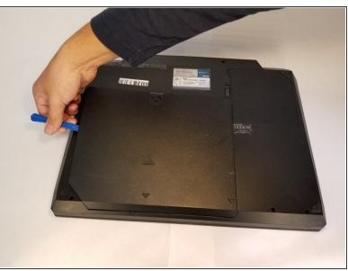
Place the device upside-down. Unscrew the screw at the top of the cover and remove the cover by using a plastic opening tool.
