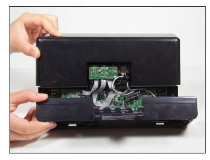
• Use your fingers or a plastic opening tool to carefully pry apart the plastic connections still connecting the base to the top.
