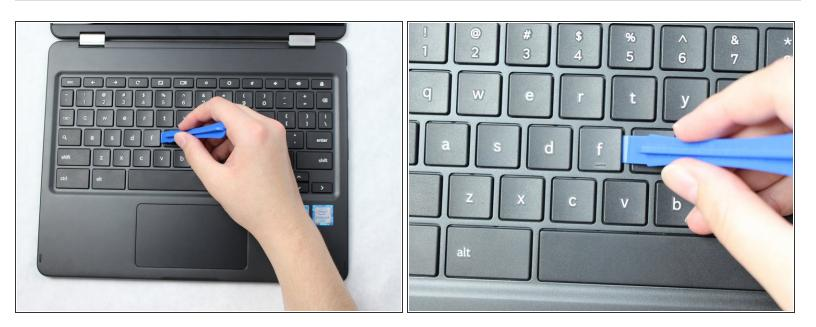
Place the plastic opening tool underneath any side of the key at an angle.
