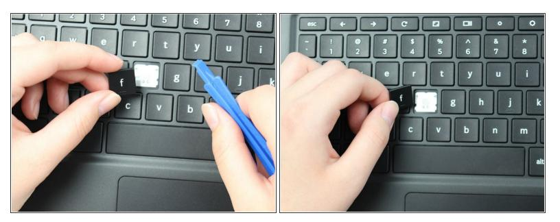
Pry the key up using the plastic opening tool.
