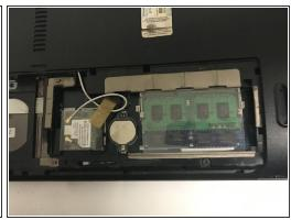
Remove the back cover by placing the plastic opening tool in the indention, and prying upwards.
