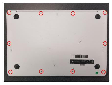
• Use a J00 screwdriver to unscrew the 10 back-plate screws.
