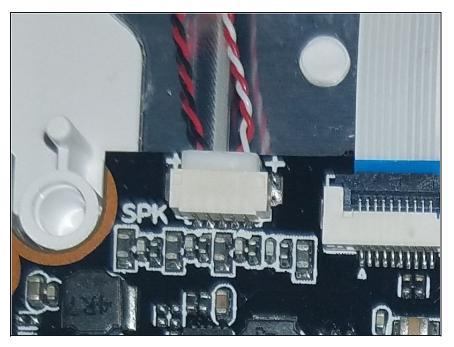
Gently pull out the speaker wire connector from the motherboard.
