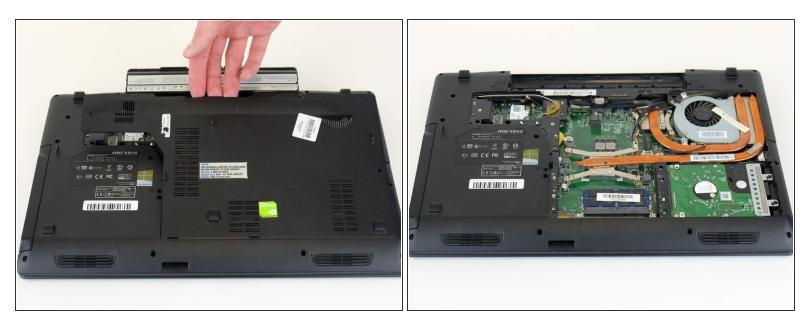
• Once all four screws are removed, lift the back off.
