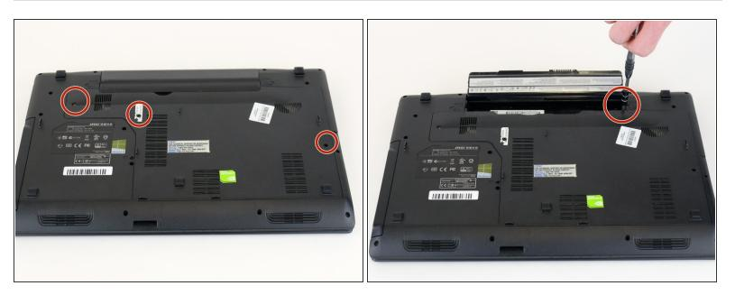
• Remove the four 5mm screws from the back of the device using a Phillips #00 screwdriver.
