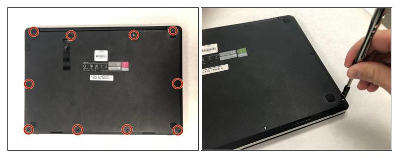
• Remove the ten 10.7 mm Phillips #0 screws from the back cover of the Asus laptop.
