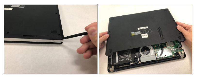
Insert the heavy duty spudger between the back cover and the laptop frame. Pull the black pry tool along the edge of the laptop, unlatching the back cover from the frame.
