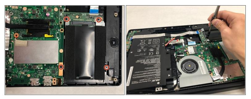
• Remove the four 4.7mm Philips #0 screws securing the hard drive.
