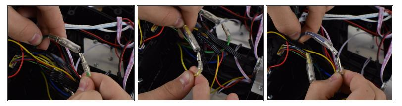
• Unplug all three of the cables that were previously zip-tied. They are the cables that are connected with a clear sleeve near the center of the device.
