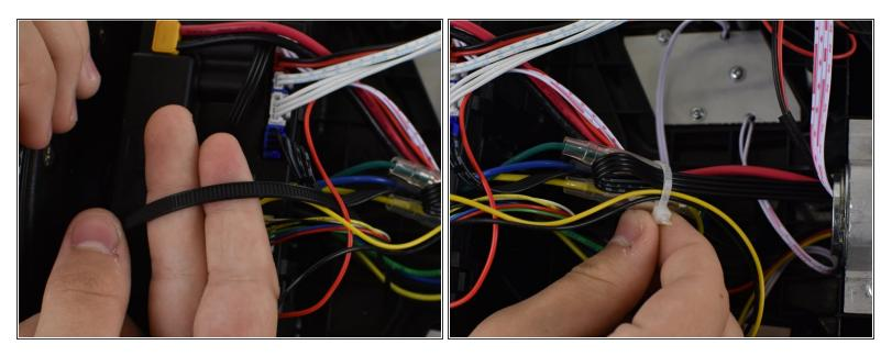
• Cut both zip-ties that secure the circuit board box and the wire bundle near the center of the device together.
