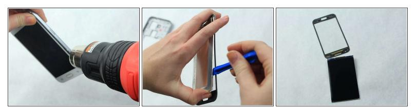
• Use a heat gun and an *iFixit Opening Tool* tool to separate the screen from the digitizer.
