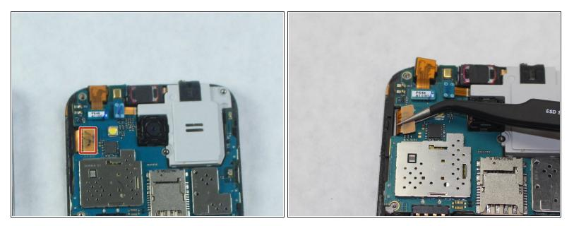
Use tweezers to disconnect the power ribbon from the motherboard.
