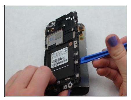
• Lift the plastic panel that separates the digitizer and the motherboard with an <u>iFixit Opening Tool</u>
