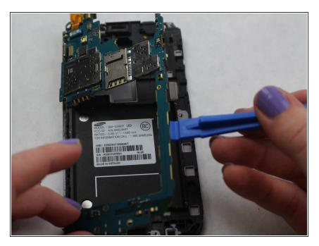
• Use the <u>iFixit Opening Tool</u> to remove the mother board.
