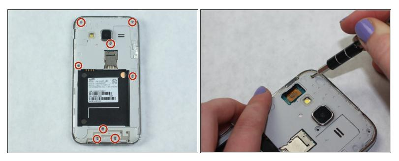
Use the Phillips #00 screwdriver to remove the eight 4 mm screws from the midframe.
