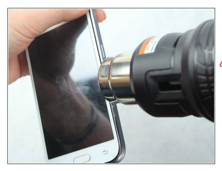
Use a heat gun or hair dryer to loosen the adhesive between the midframe and the rest of the device.
