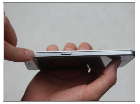
• Turn the smartphone off by using the power button on the right-hand side.
