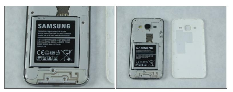
• Locate the battery near the bottom of the phone. The battery is square, flat, and is labeled 'SAMSUNG'.
