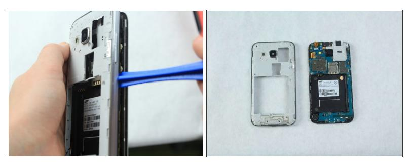
• Use the *iFixit Opening Tool* to lift the frame.
