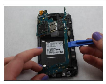
Lift the motherboard out using the <u>iFixit Opening Tool</u>.
