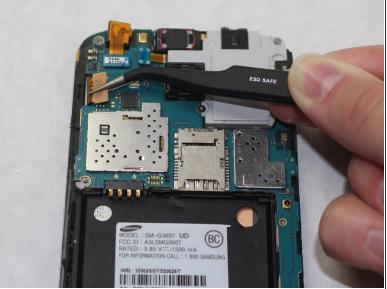
Disconnect the LCD screen/touch screen ribbon from the motherboard using tweezers.
