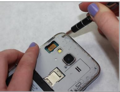
Use a Phillips #00 screwdriver to remove the eight 4 mm screws that secure the midframe.
