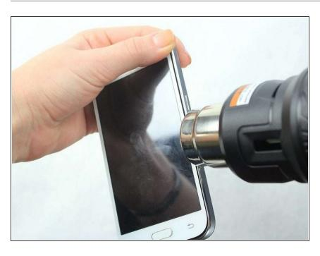
Heat the sides of the screen with a heat gun or hair dryer.
