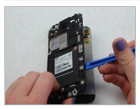
Use the <u>iFixit Opening Tool</u> to remove the plastic panel that separates the motherboard and the screen.
