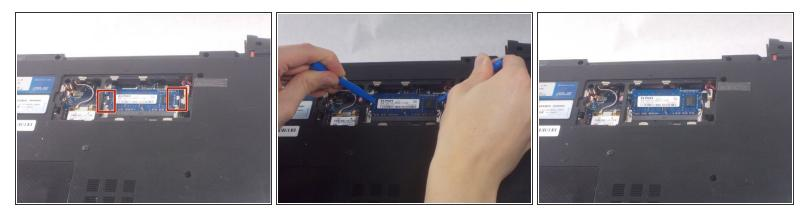
• Use plastic opening tools to move the metal clips holding the RAM in place outwards.
