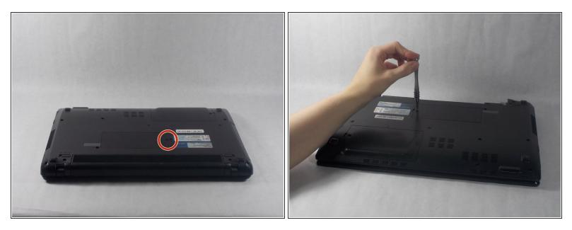
• Remove the 5mm screw holding the RAM panel in place with a Phillips #1 screwdriver.
