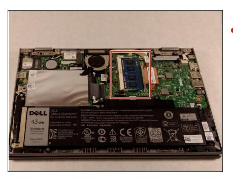
Locate the RAM chips on the motherboard.
