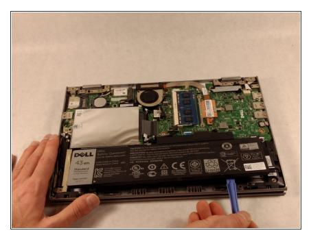
Using the iFixit opening tools, lift the battery out of its housing.
