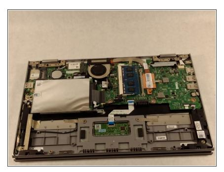
Remove the battery completely.
