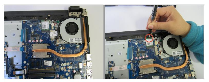
• Use a Phillips screwdriver to remove the screw holding down the wifi chip.
